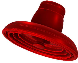
Fig. 3. Three-dimensional model of the suspension glass insulator.
